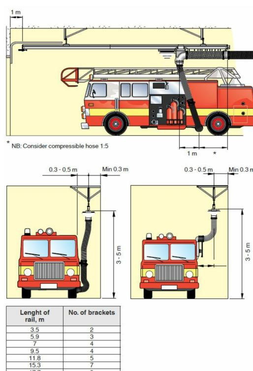
N.B. The nozzle for high level (HL) exhaust pipes must be installed at a higher level than the exhaust pipe. The nozzle must be pulled downwards at connection, which will activate the balancer.
